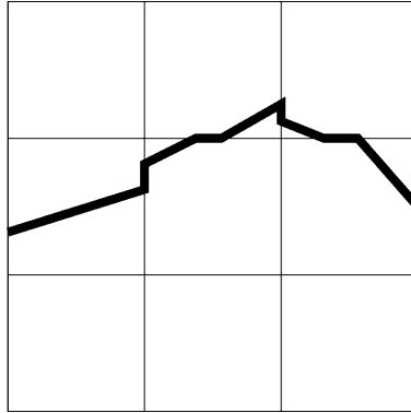
Fig. 9. The volume-of-fluid reconstructed interface consists of the piecewise linear line segments along with the portions of the cell boundaries that make up the difference between neighboring line segments. This is an exaggerated diagram. The magnitude of the discontinuity between neighboring segments is O(\Delta x^2) .
